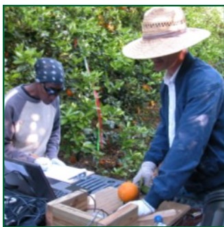
Pull-test measurements help to determine the loosening effect abscission applications have on citrus trees prepped for mechanical harvesting.
